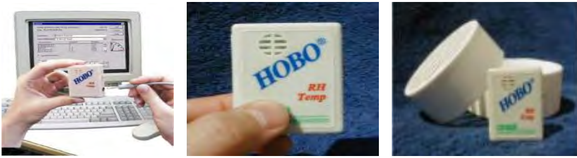
Fig 1: THI logger system
